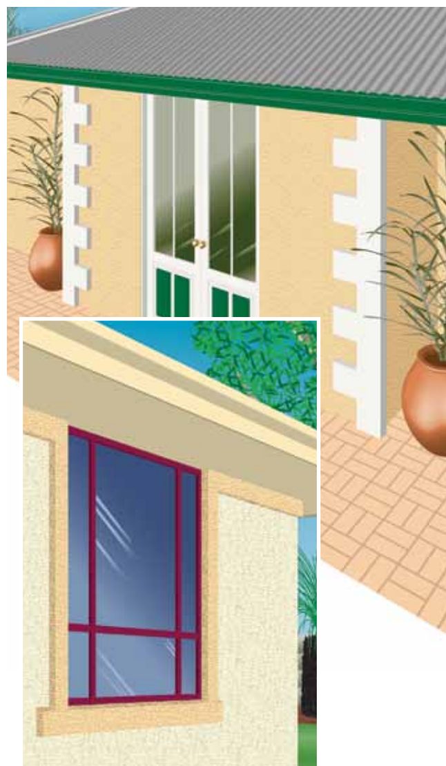
Corbelling and Projecting Sills provide effective highlighting for corners, windows and eaves
