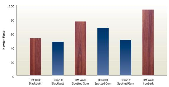
The dint test is the amount of force required to put a dint into the surface of the product. A higher number represents more force is required to dint the surface.
