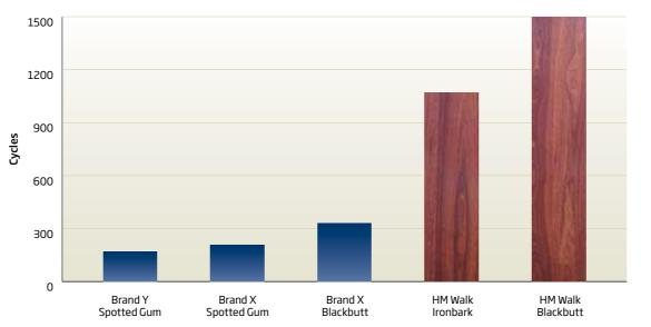
The abrasion test uses an abrasive on a wheel and measures the number of cycle revolutions that is required to wear through the coating to bare wood. The higher the number of cycles the more abrasive resistant the coating is to wear.
