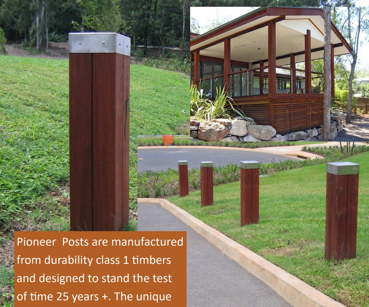
Pioneer Posts are manufactured from durability class 1 timbers and designed to stand the test of time 25 years +. The unique profile is designed with expansion joints which work in the same manner as concrete to eliminate unsightly cracks as the timber dries out. A stainless steel cap is optional and can be fitted to stop water penetration into the end grain to ensure longevity. Pioneer bollards are extremely strong and suitable as ram raid barriers.
