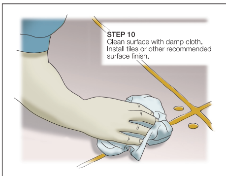
FIGURE 11 CLEANING SURFACE FOR WET AREAS
