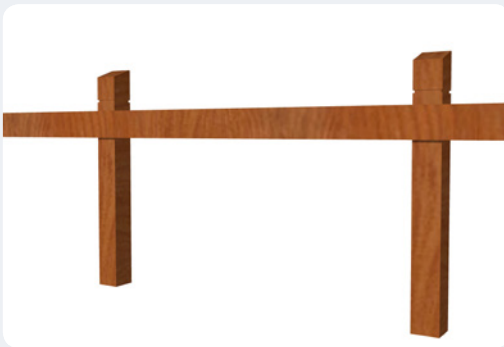
F: Recessed rails – Rebates for rails offer better support, though greater potential for decay.
