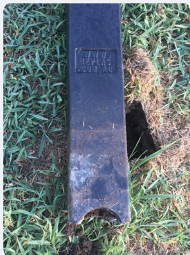
A: Sheared bollard – This new recycled plastic bollard was sheared at the ground by vehicle impact.
