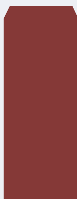
B: Built top rail profile – A flat-topped member with arrissed edges was installed.
