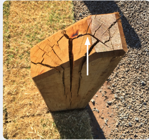
B: Splitting in an arc on the heart and heartwood border
