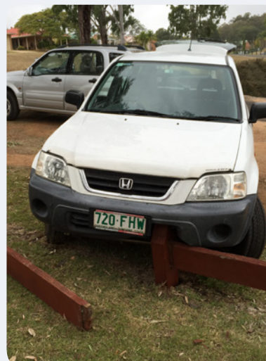
C: Hardwood barrier – The 30-year-old hardwood barrier is shown here intact despite having rendered considerable damage to the vehicle.
