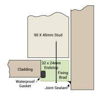
\* 9mm x 1.6mm gaskets are factory fitted. Additional foam gaskets, to form second moisture barrier, are available in rolls for on-site installation, or alternative sealant method can be implemented.
