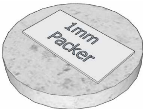
Insulating packer or similar provide barrier between concrete and aluminium bracket
