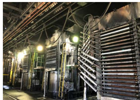
The hot press ( where all moisture is taken out of the sheets )
