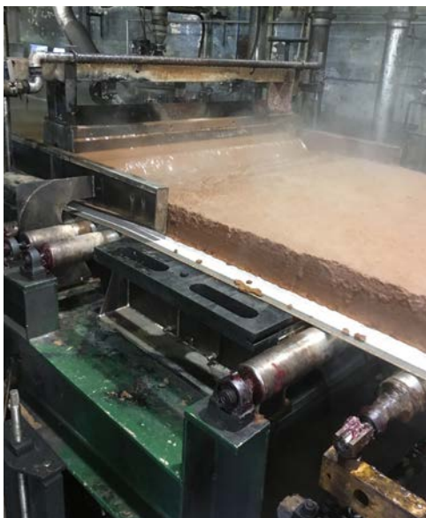
Pulp getting made into board ( These 'slabs of pulp' will be rolled and pressed to produce a 9.5mm board/sheet )
