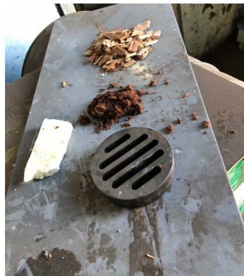
The woodchip gets blasted through this 20cm grate and cooked via 900 psig of saturated steam in the mason gun. What is left is a tobacco looking substance. Paraffin wax is then added.
