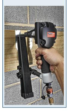
In case you haven't heard, the Collated Connector Nailer is a pretty handy piece of kit to have on the job site. It will precisely install connector nails faster than nailing by hand. It is more precise than a standard nail gun because it protrudes the nail it is about to drive from the tip of the tool. This means that you can precisely locate each and every hole.
