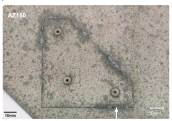
Dark areas indicate metallic coating corrosion originating from the cut-edge.
